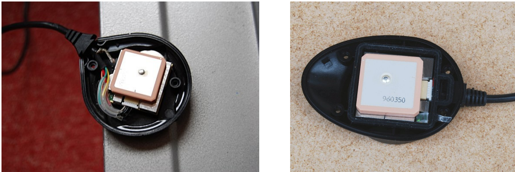
Figure 58: An EM-406A module embedded into the housing of a Fortuna U2/PS2, to the left, and embedded into a housing of a Navilock NL-303P, to the right
