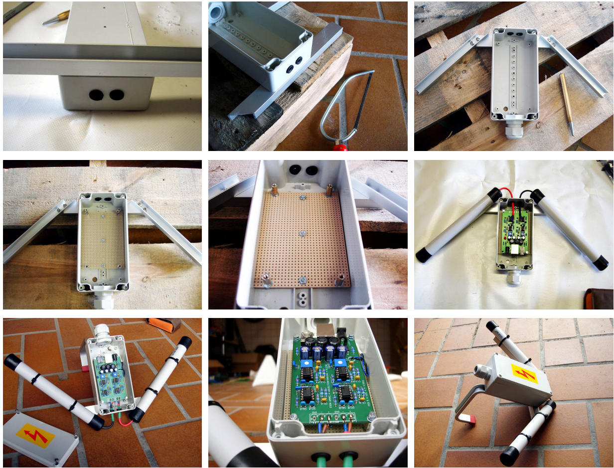
Figure 20: A guidance for building an outdoor ferrite rod antenna, continued, ©Florian Bamberg
